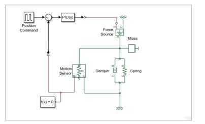
The control Simulink signal goes to the input port of the Simulink-PS Converter block, where it is converted into a physical signal driving the force profile of the Ideal Force Source block.
